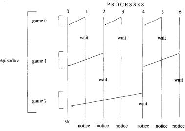
Fig. 5. Communication structure for the tournament algorithm.
