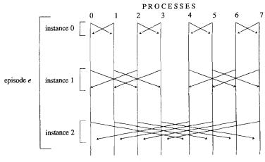
Fig. 3. Communication structure for Brooks' algorithm.
