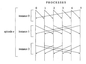
Fig. 4. Communication structure for the dissemination algorithm.
